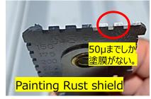
"During application, we always verify that the film thickness is 75µm with a film thickness gauge. If it's too thin, we instruct for a recoat."
